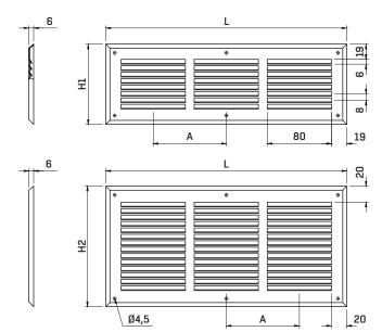
Installing hole: L-36 x H1 - 36 H2 - 36
