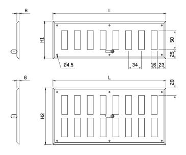
Installing hole: L-36 x H1 - 36 H2 - 36
